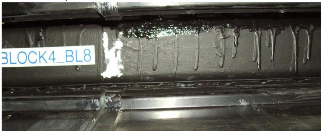
Figure 25: Black paint and RTV adhesive on Modules.
