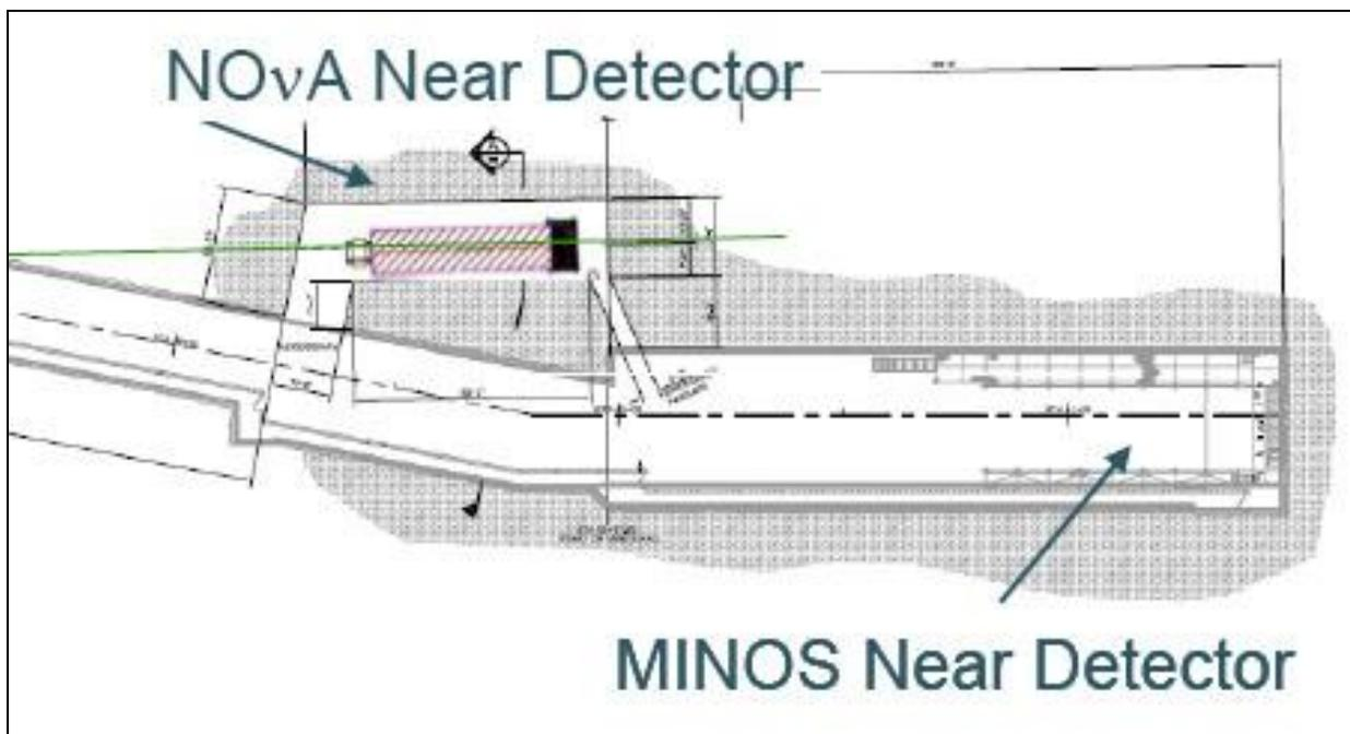
Figure 4: The NOvA Near Detectors in a cavern adjacent to the MINOS access tunnel.
