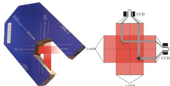
Figure 5: XLS Measurement principle
