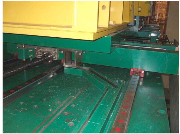
Figure 15: Rail for rolling the BELLE detector in and out.
