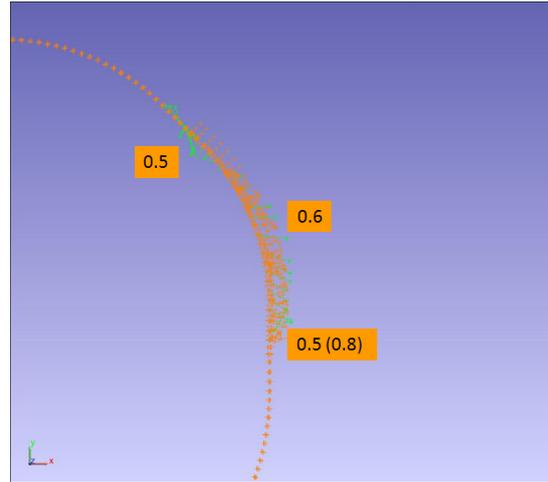
Figure 7: Comparison between prediction of model C and measurements from 3<sup>rd</sup> epoch, values in mm
