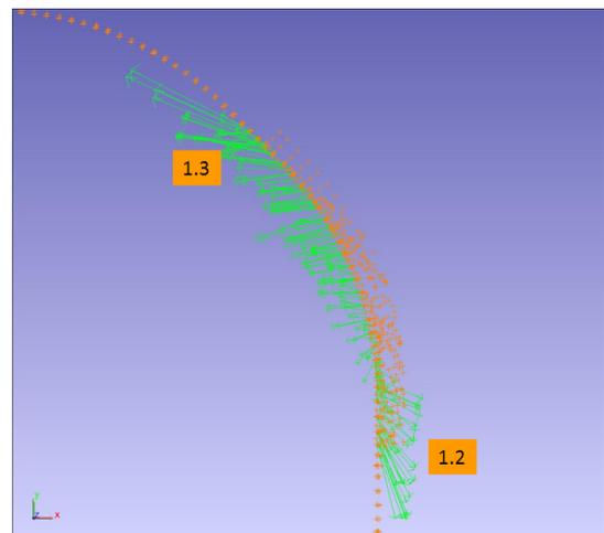
Figure 8: Movement of floor monuments between 3<sup>rd</sup> and 4<sup>th</sup> epoch, values in mm
