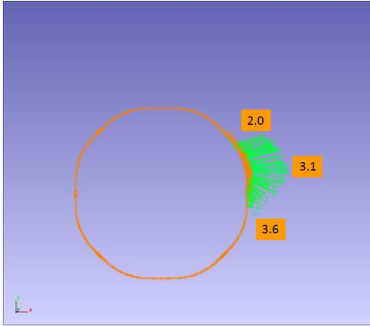
Figure 5: Comparison between prediction of model A and measurements from 3<sup>rd</sup> epoch, values in mm
