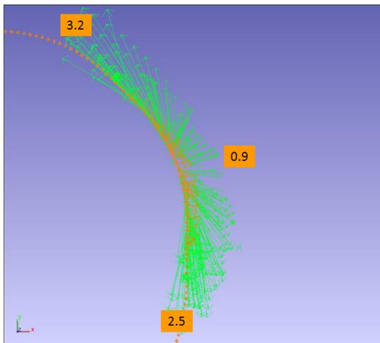
Figure 6: Movement of floor monuments between 2<sup>nd</sup> and 3<sup>rd</sup> epoch, values in mm
