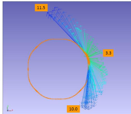
Figure 4: Movement of floor monuments between 1<sup>st</sup> and 3<sup>rd</sup> epoch, values in mm
