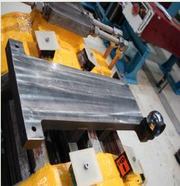
Fig. 2 Specially designed alignment adapter for Booster corrector magnets
