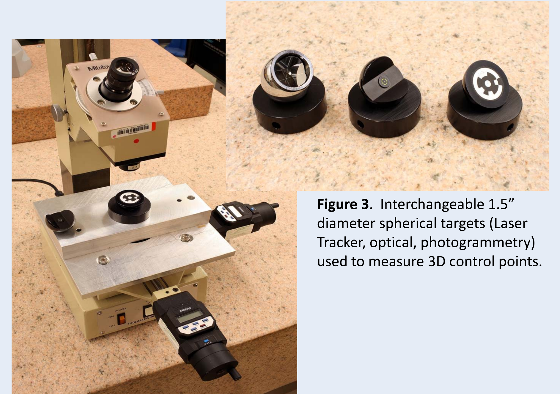
Figure 2. Tooling microscope with special fixture used for in-house production of RAD coded spherical targets compatible with Laser Tracker and optical targets.
