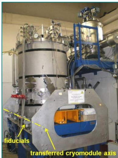
Figure 8: Cryomodule B on the bench for axis transfer operation
